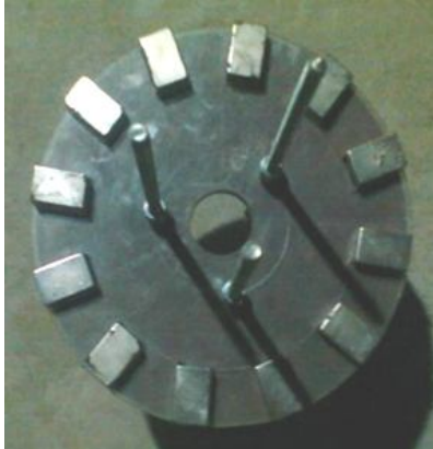
Fig. 4. Rotor assembly with permanent magnet.
